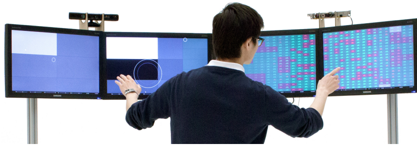
Figure 1: A user is standing in front of the Perifoveal Display. Two depth cameras track the user's head direction. At the focal point more detailed information is shown. The data becomes increasingly abstracted the further away it is from the user's focus. In the periphery changes in brightness and movement indicate changes in the data and these can be perceived by the user.
